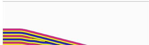
Ply drops and embedded delaminations
